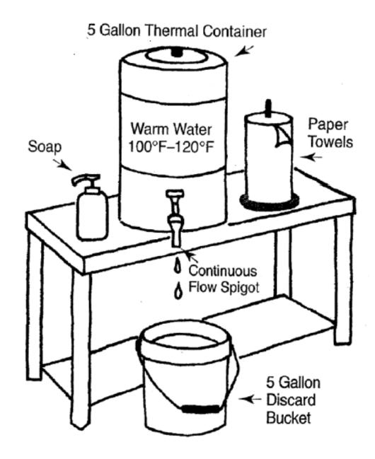
The container holding the water must have a spigot valve that allows continuous free flowing of water to properly wash your hands.
